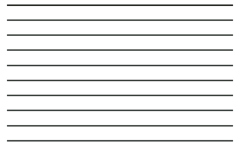
Fig. 9.45 - The single line has been duplicated to form a series of 10 lines, 4mm apart using: No of times = 9 , Vertical offset = 3mm , Horizontal offset = 0mm .
