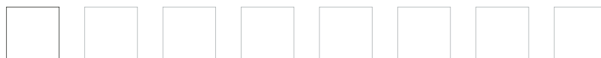
Fig. 9.46 - The single 10mm x 10mm frame has been duplicated to form a series of 8 frames, 5mm apart using: No of times = 7 , Vertical offset = 0mm , Horizontal offset = 15mm .
